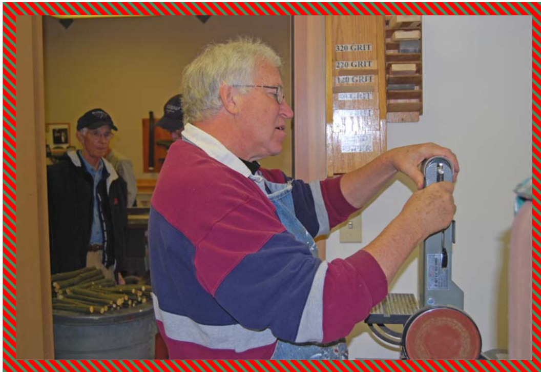
Dan Holtz replaces a worn sanding belt.
